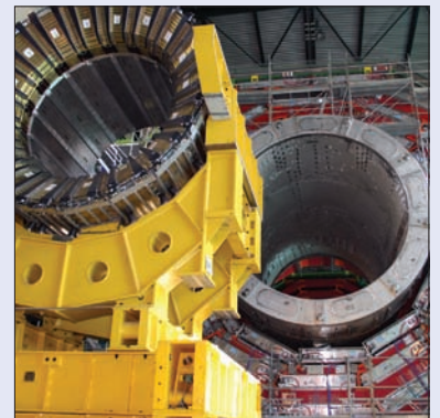
The first half of the barrel hadron calorimeter was tested in March 2006 using a radioactive source before insertion into the solenoid in early April. The second half was inserted a month later.
