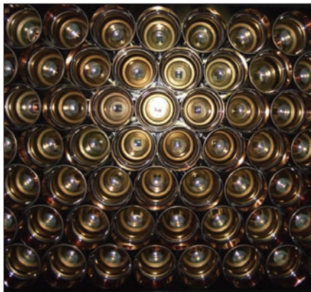
HPDs mounted in the LHCb-RICH detectors Photograph courtesy of R. Plackett/ Imperial College London
