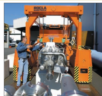
More than 80 dipole cold masses had arrived at CERN by late summer 2003. This one is being installed in the robotic "crab", designed to carry the magnets around the site.
