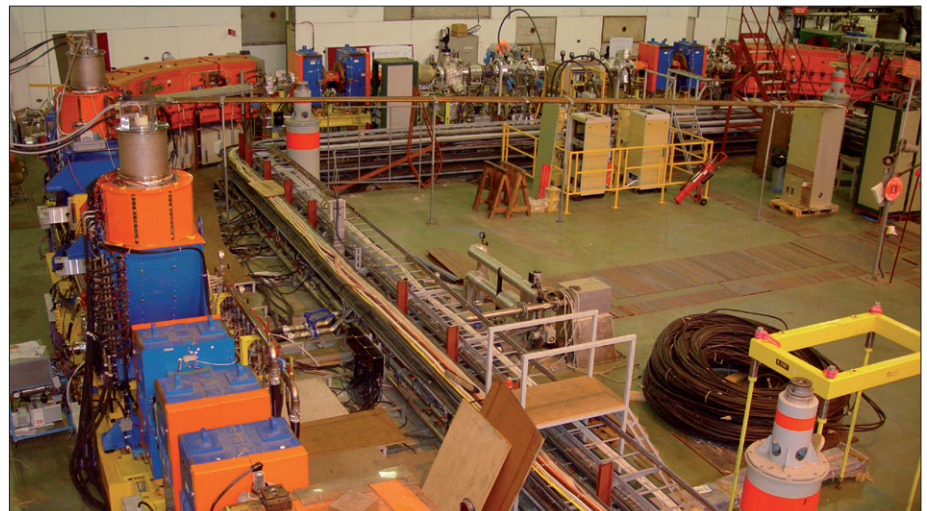
Figure 2. View of the Low Energy Ion Ring with its electron cooler on the left (courtesy of CERN).
