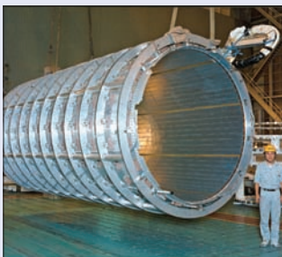
The coil winding for the central solenoid magnet was completed in Japan in 1999. The superconducting magnet provides a field of 2T at the centre of ATLAS's tracking volume.
