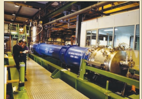
In April 1994 the first LHC dipole prototype was successfully powered for the first time.
