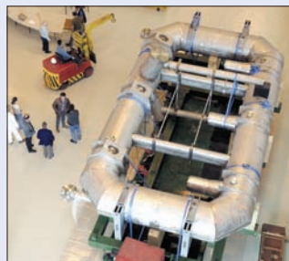
The prototype B-0 toroid coil arrived at CERN from the CEA laboratory in Saclay on 6 October 2000. At "only" 9m in length this prototype is the largest toroid coil ever built.
