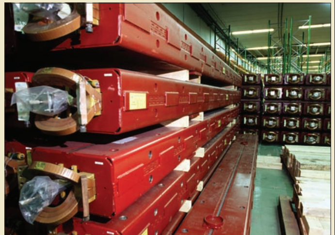
The Budker Institute of Nuclear Physics in Novosibirsk supplied some 540 magnets for the transfer lines from the SPS to the LHC, as part of the Russian contribution.
