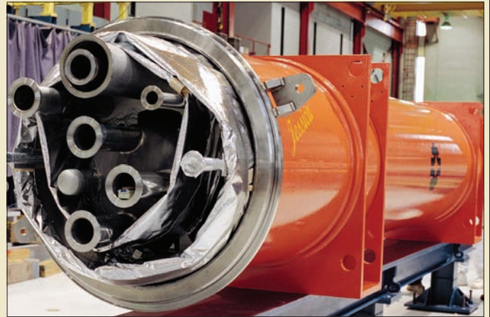
A prototype superconducting quadrupole magnet for the interaction regions at the LHC under assembly at Fermilab. Similar magnets are also being supplied by Japan.
