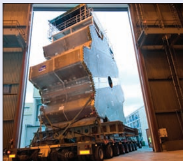
Moving at 1 km/hour on a special trailer the first of the endcap toroids leaves the assembly hall in February 2007 before being cold-tested at 80 K, prior to installation in the cavern. ● March 2007 p6.
